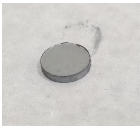
Figure 21: an SnS pellet synthesized by method 1.
