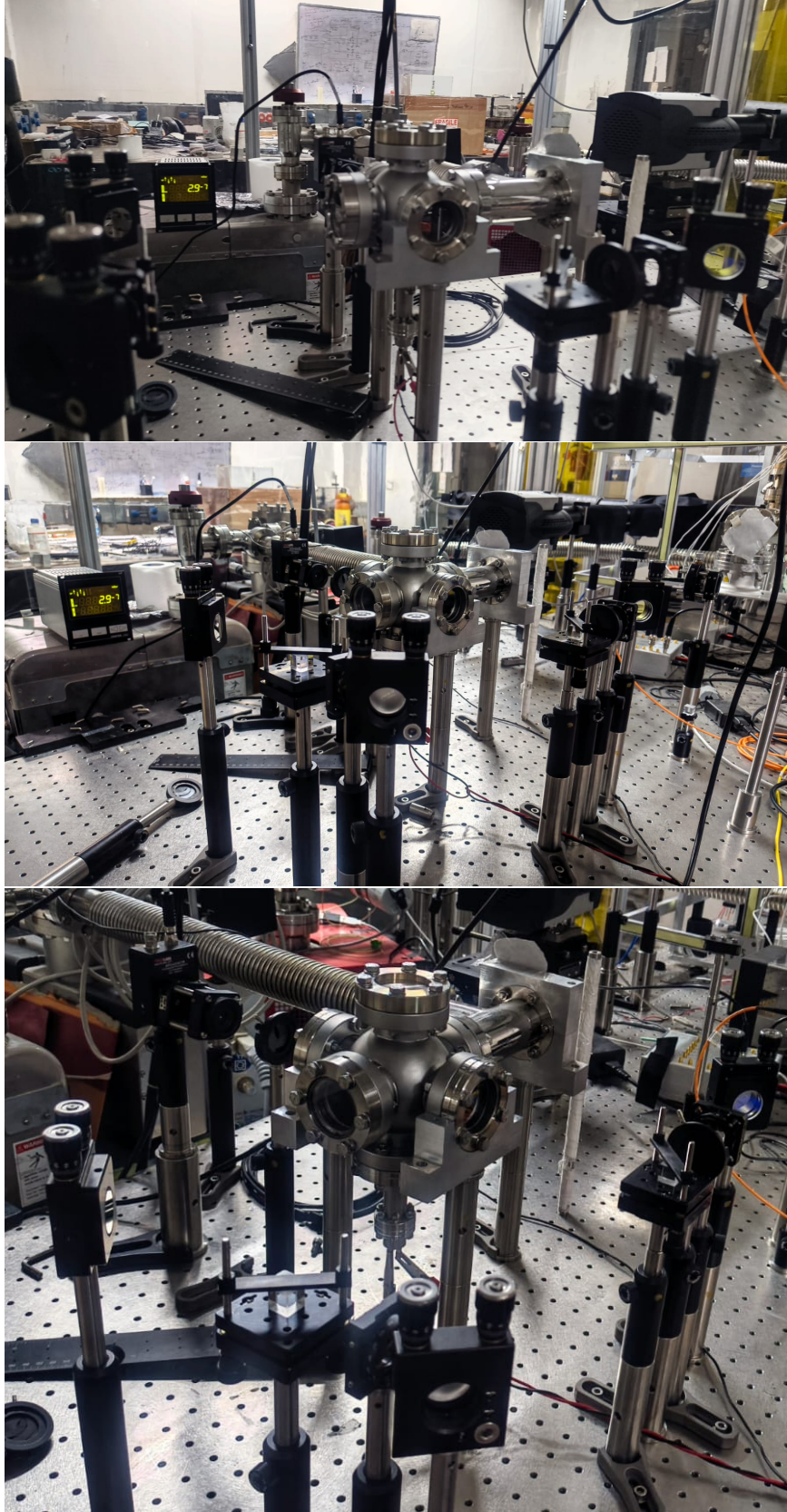
Figure 1.5: Photographs of the assembled experimental apparatus from multiple angles, showing the vacuum chamber, optical mounts, mirror alignment stages, and detector assembly.
