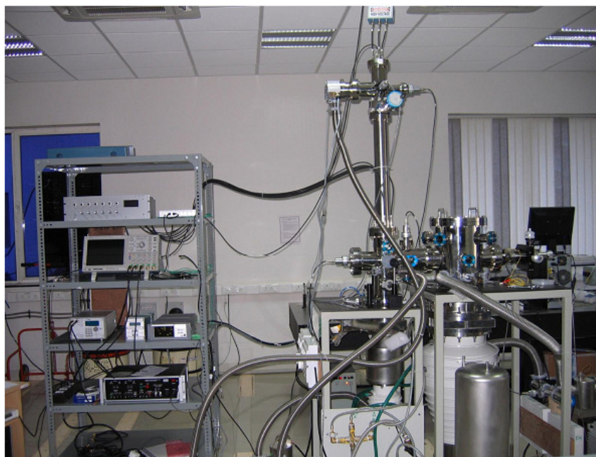
Figure1. Picture of home-built REMPI Time Of Flight Mass spectrometer
