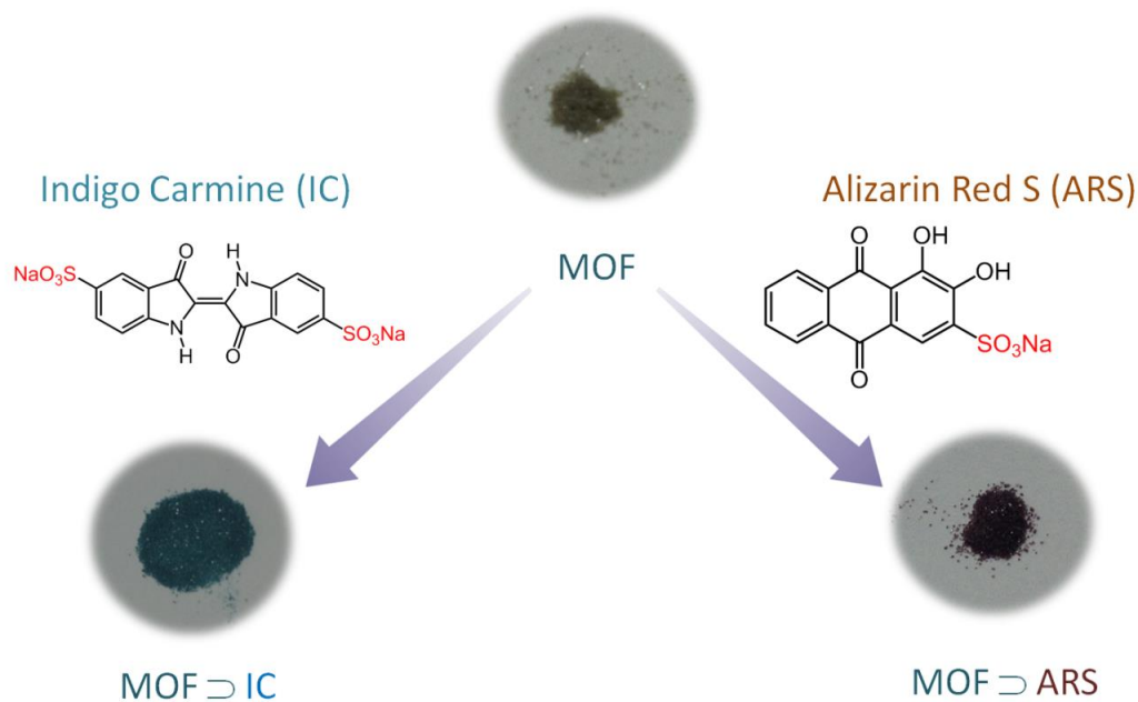
Appendix 5.49: Illustration showing capture of anionic dyes (IC & ARS) by compound IPM-MOF-201 .
