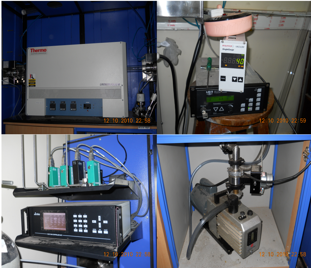
Figure 3.1: The experimental set up for the CVD growth of graphene . The furnace, pressure gauge, vacuum pump with butterfly valve, MKS mass flow controller (in clockwise order from the left top).
