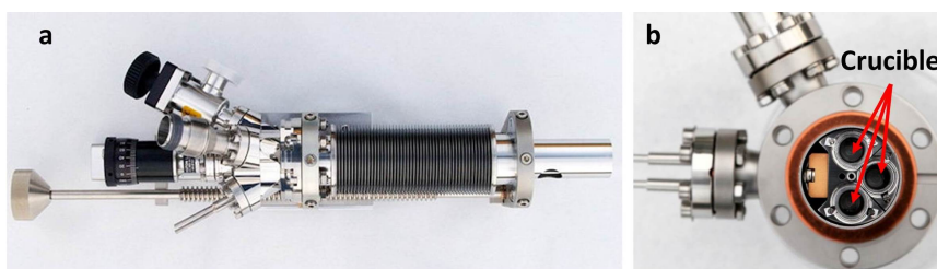
FIGURE 2.8: a) Actual picture of the molecule evaporator. b) Inside view of the crucibles. Three crucibles are marked with red arrow. They are thermally isolated from each other.
