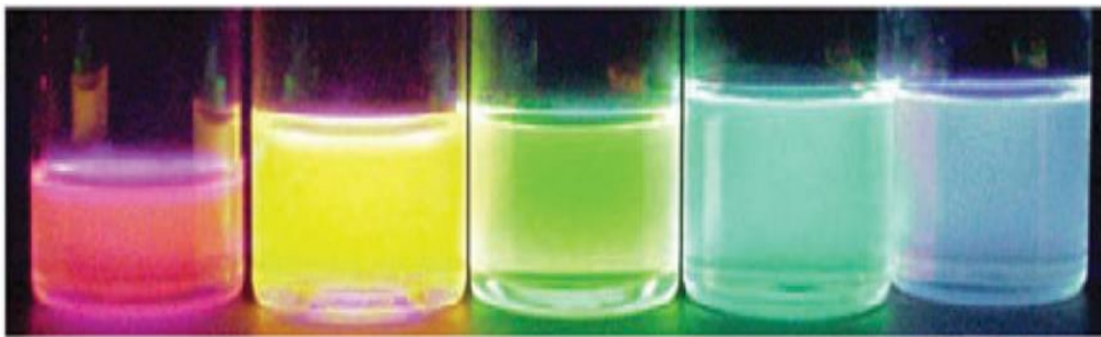
Figure 1.3: Color tunability. Photograph of UV-light excited colloidal solution of CdSe QDs with different sizes. PL color changes from red to blue as QD size is reduced from 6 to 2 nm. Reprinted with permission from Ref.11. Copyright 2011, Royal Society of Chemistry.
