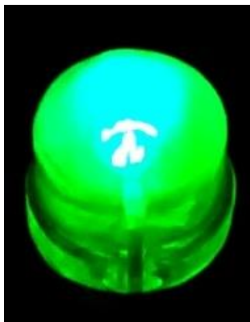
Figure 3A.8: CsPbBr 3 nanocrystals as emitter. Photograph of a green LED obtained after coating an UV-LED with CsPbBr 3 nanocrystals.
