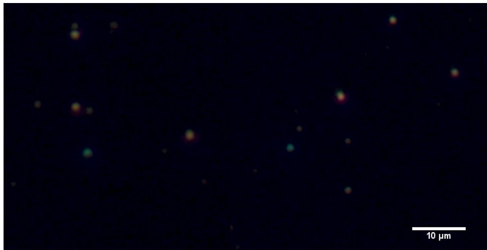
Figure 4.5: Gold Nanoparticles under Dark field illumination
