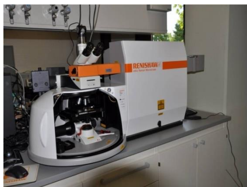
Figure 13: Raman microscope and instrumentation
