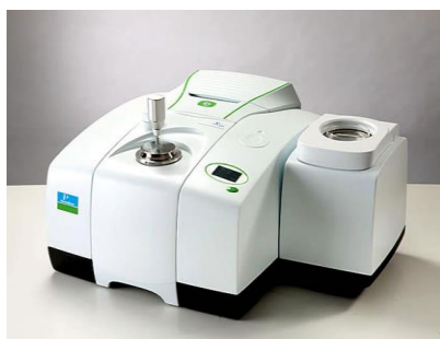
Figure 12: Fourier transform infrared spectrometer. Principle of working – Michaelson interferometry
