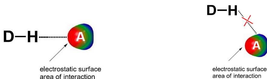
Fig 1: Hydrogen bonding between the acceptor (A) and the hydrogen atom of the donor (D). The directionality of the (head-on or end-on binding, not side-on binding) electrostatic surface dictates the directionality of the hydrogen bonding which is not observed on the right resulting from an acute bond angle and where there is no contact with the electrostatic potential area of interaction (shown in red in potential map).
