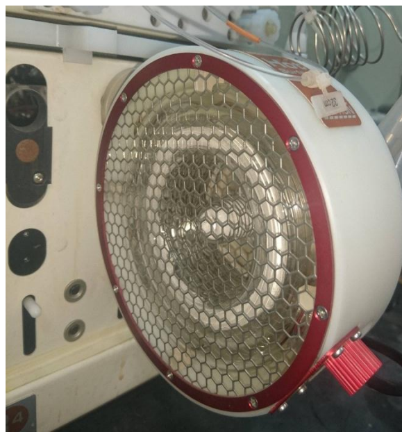
Figure 3A.1. (a) The full setup for the Vapourtec R-series reactor from our laboratory; (b) Image for the coiled reactor.
