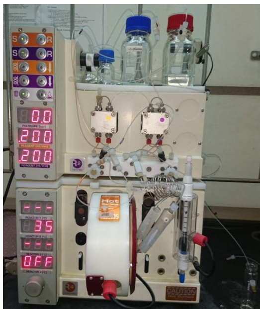
Figure 3A.1. (a) The full setup for the Vapourtec R-series reactor from our laboratory; (b) Image for the coiled reactor.
