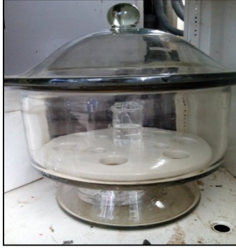
Figure 1: Reaction vessel for synthesizing \text{CaCO}_3 by room temperature carbonation process.
