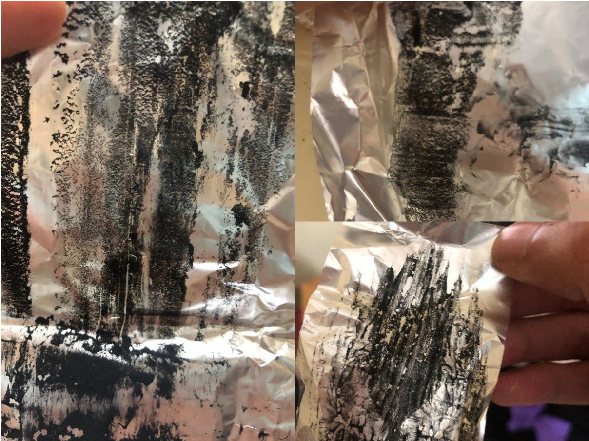
Fig.3.6 Non homogeneous slurry after coating on the sheets.
