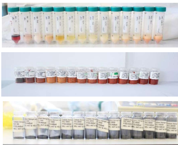
Figure 21: From top to bottom: Xerogels in suspension (R/C 50 -R/C 20000 ) and powder form and Xerogels after carbonization ( C_{XGs} )
