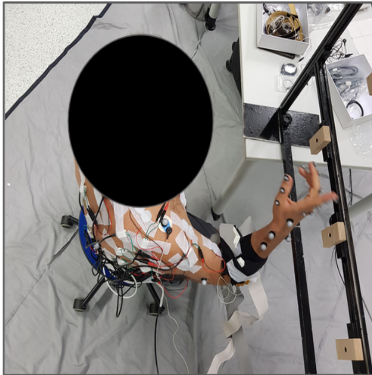
Figure 3.3: Subject (anonymized) performing the grasping task with the EMG electrodes and motion capture markers attached.
