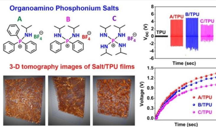
Figure 4: Organoamino phosphonium salts and their polymeric composite materials for mechanical energy harvesting applications.
