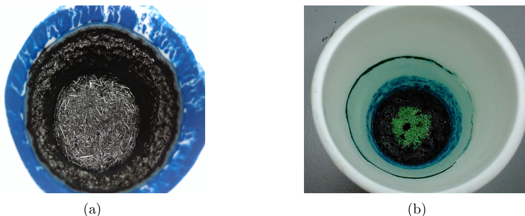
Figure 2.1: Photos of sample after reaction (a) \text{Co}_2\text{AlO}_2\text{BO}_3 after reaction (blue color sample stick to the walls are cobalt oxides which was washed out by HCl) (b) \text{Ni}_2\text{AlO}_2\text{BO}_3 after reaction (green patch in center is nickel oxide)
