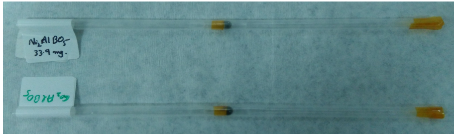
Figure 2.3: Sample holder with plastic straw and capsule filled with powdered sample
