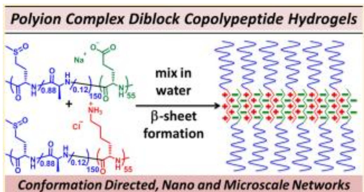
Figure 1.16. Schematic representation of two oppositely charged diblock copolymer followed by their polyion complexation. (Adopted from Deming and coworkers. J. Am. Chem. Soc. 2017 , 139 , 15114–15121)
