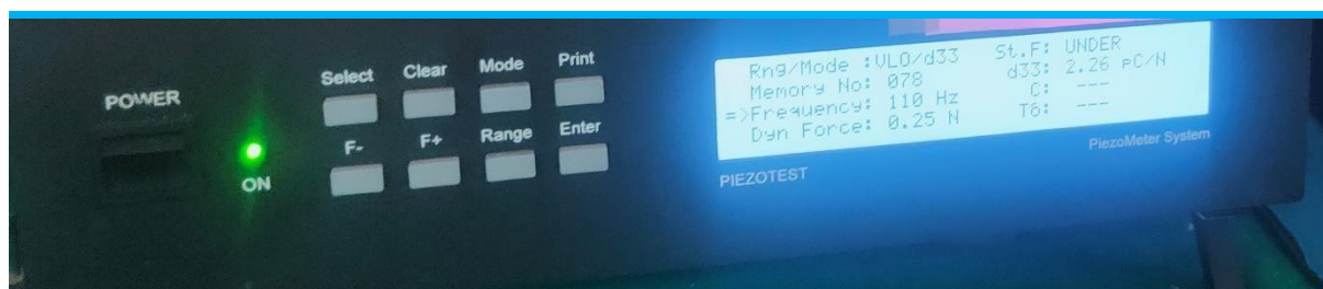
Figure A16: Photograph of the displayed d_{33} measurement details of 2 in piezometer.
