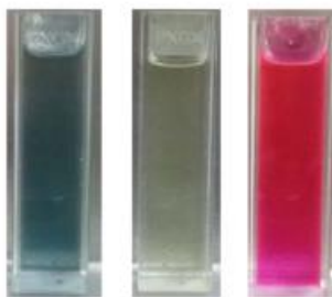
Figure 5.4 Demonstrating the optically excited blue, green and red carbon dots dispersed into ethanol under UV excitation.
