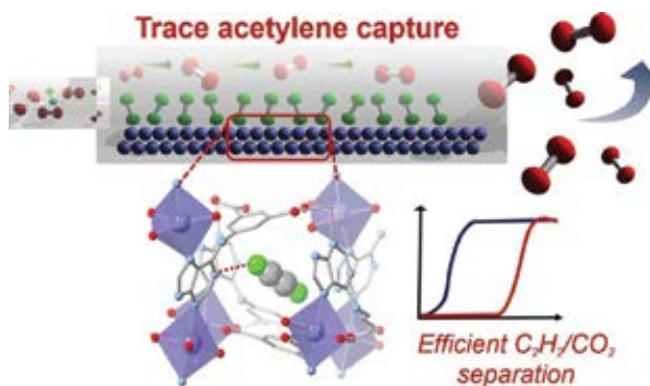
Figure 6: Efficient capture of trace acetylene by an ultramicroporous metal–organic framework (MOF) (Prof. Sujit Ghosh's Group)
