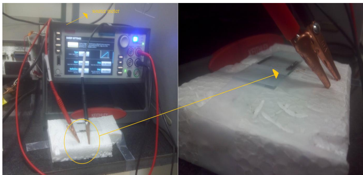
Fig 3.11 : (a) I-V measurements were done using source meter. (b) inset: Co@CNTs were dropcasted between two gold electrodes.
