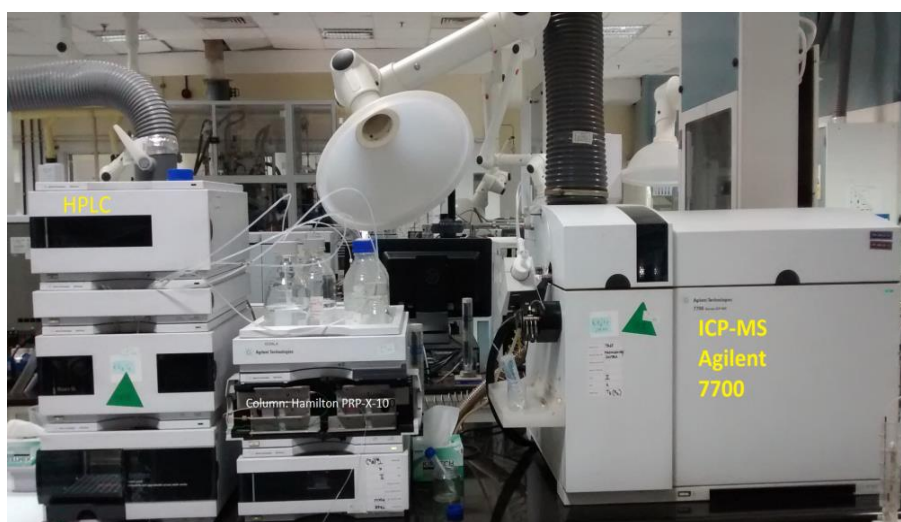
Fig. 4: Schematic presentation of the hyphenated system of HPLC and ICP-MS
