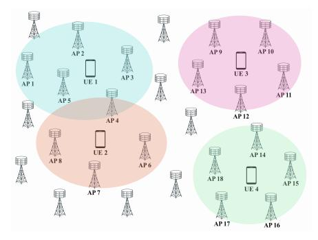
Figure 4: AP selection in cell-free massive mMIMO system
