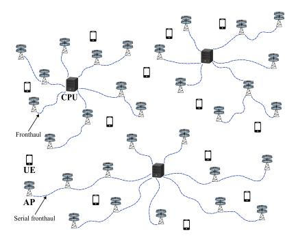
Figure 3: Schematic diagram of Cell-free network architecture
