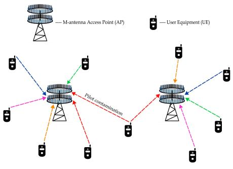
The different coloured arrows represent orthogonal pilot signals from user terminals to access points for uplink channel estimation.
