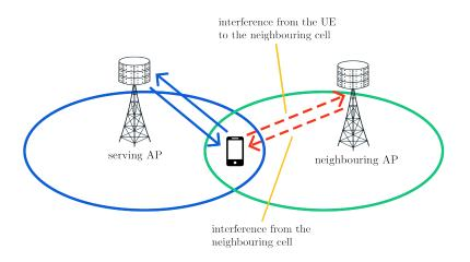
Figure 2: Schematic representation of inter-cell interference
