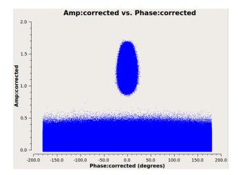
Figure B.3: Amplitude and Phase for the Gain calibrator in the MS for IRAS 11119+3257. The gain calibrator is a point source and is expected to have a confined oval centred at the known amplitude with a small spread in phase in the plot. We can see that while this is true, there is some 'bad data' that spreads below the oval. The data points were identified and flagged.
