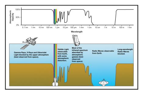
Figure 2.1: Atmospheric Electromagnetic Transmittance shows that the optical wavelengths are affected by the atmosphere, and IR wavelengths have no transmittance. The radio wavelengths are not obstructed by the atmosphere. *Image credits: NASA*
