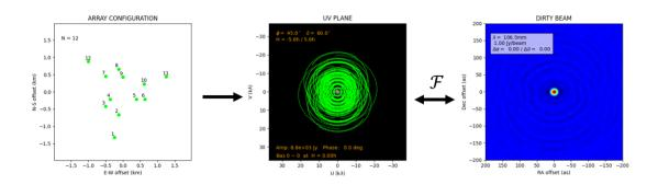
Figure 3.1: Each antenna pair measures visibility in the UV plane. The Fourier transform of the measured visibilities is the Point Spread Function (PSF) or the Dirty Beam of the antennas. *Image Credits:* APSYNSIM[21]
