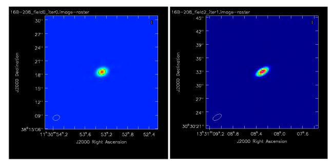
Figure B.1: The images of the calibrators are plotted. The image of the flux calibrator on the right shows that it is a compact source. The flux we should get is 14.6 Jy [43]. The flux density obtained is 14.3 Jy. This is very close to the expected value. The image of the Phase Calibrator shows that it is a compact source. The flux density of the phase calibrator from fluxscale should be around 1.2 Jy. The flux extracted is very close to the value given by fluxscale.
