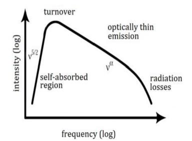
Figure 1.8: A generic synchrotron spectrum Image Credits: Multifrequency study of GHz-peaked spectrum sources and candidates with RATAN-600 radio telescope, Group IAG
