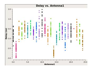
Figure B.4: The delay solutions for IRAS 11119+3257 is plotted as a function of antennas. The delays are expected to be less than 4 ns for the upgraded VLA, which is seen in the plot
