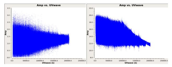
Figure B.2: The Amplitude vs UV-Distance Plots for the calibrators are plotted. Both the Flux (on the right) and Gain calibrator (on the left) seem to show constant amplitude for shorter baselines like point sources and then show a steep drop in amplitude like extended sources at larger baselines
