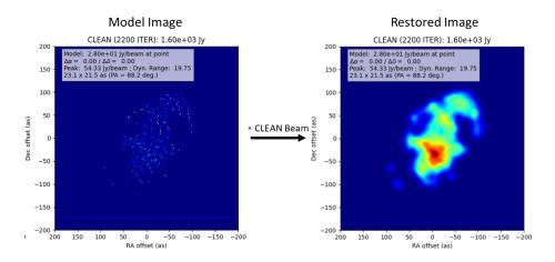
Figure 3.4: The model sky image is convolved with an Ideal PSF or the CLEAN Beam to get a CLEAN Restored Image. *Image Credits:* APSYNSIM[21]
