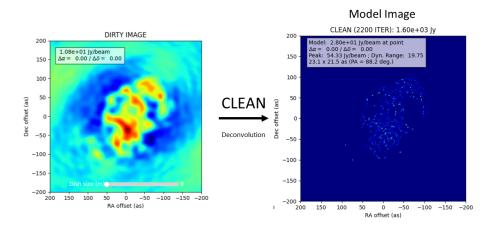
Figure 3.3: The Dirty Image is deconvolved or CLEAN-ed to get a Model Sky Image, a collection of delta functions of the brightest pixels in the Dirty Image. *Image Credits:* APSYNSIM[21]
