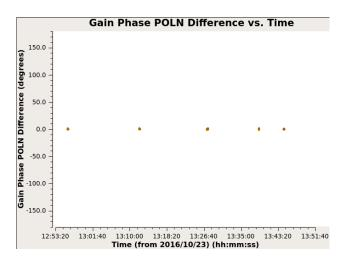
Figure B.7: The plot is the ratio of gain phase solutions of the two polarisations for the chosen reference antenna. The phase stability of the reference antenna, i.e., to have a constant phase difference between the polarisations with time, can be tested. As the plot is relatively flat, we conclude that the chosen reference antenna is stable.
