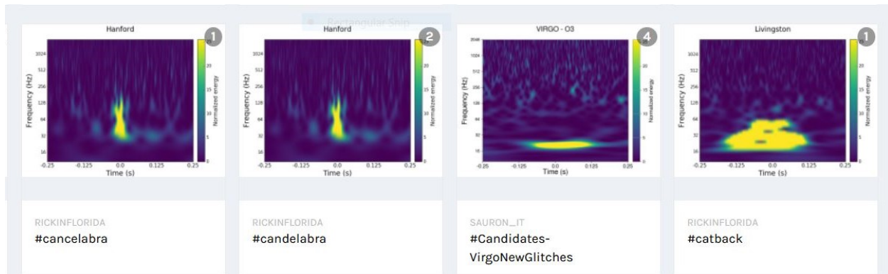
Figure 1.4: Glitches present in data from the LIGO Hanford, LIGO Livingston and Virgo detectors from the Gravity Spy gallery [17].
