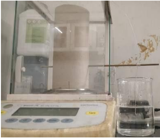
Fig 2.7: a) Archimedes setup and b) Top view of the sample holder immersed in the IPA
