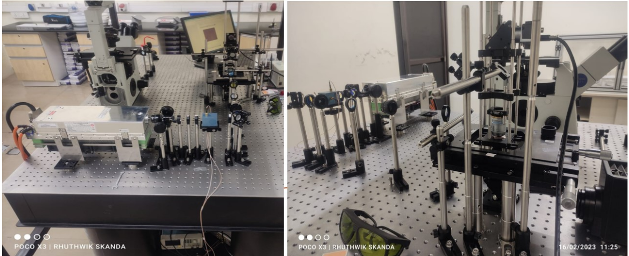
Figure 3.9: Experimental Setup for time shared optical traps setup using 2axis AOD
