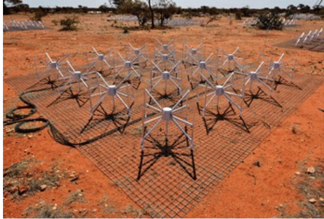
Figure 1.2: A typical MWA tile consisting of 16 phased dipoles. Image credits : http://www.caastro.org/news/tingay-et-al-pasa-2013
