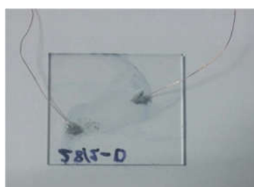
Figure 3.19 : Slide prepared for conductivity measurements on thin film
