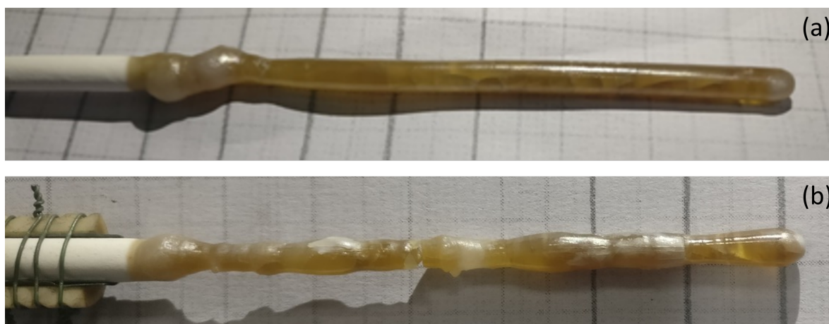
Figure 6.7: (a) and (b) show the representative images of the crystals of \text{Ca}_3\text{MgNb}_2\text{O}_9 grown at 5 \text{ mm h}^{-1} and 2 \text{ mm h}^{-1} respectively in flowing air atmosphere.
