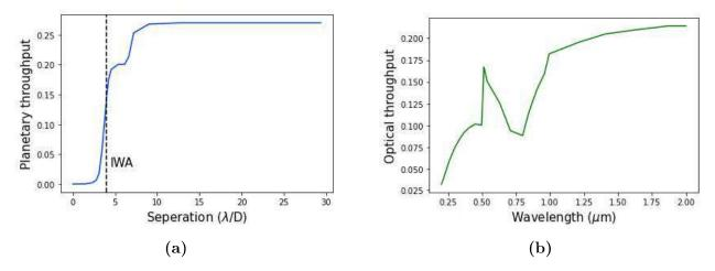
**Figure 3.3:** (a) Planetary and (b) Optical throughput of the coronagraph for the LUVOIR-A mission concept.
