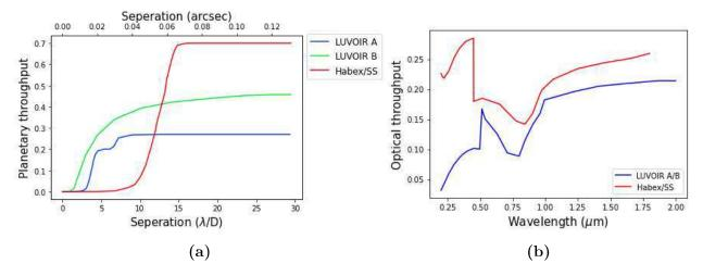
**Figure 10.1:** The (a) planetary throughput as a function of separation and the (b) optical throughput as a function of wavelength for the different mission concepts.
