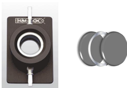
Figure 2.8. A typical sample cell for liquid samples where the sample is injected between the two windows separated by a spacer.
