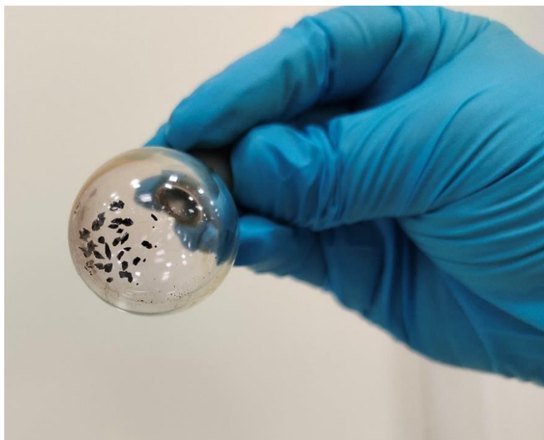
Figure 5.21: Digital image of recovered solid molecular Iodine.
