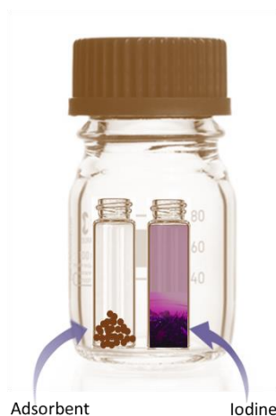
Figure 5.2: Schematic diagram of the experimental setup for vapour phase static \text{I}_2 capture.
