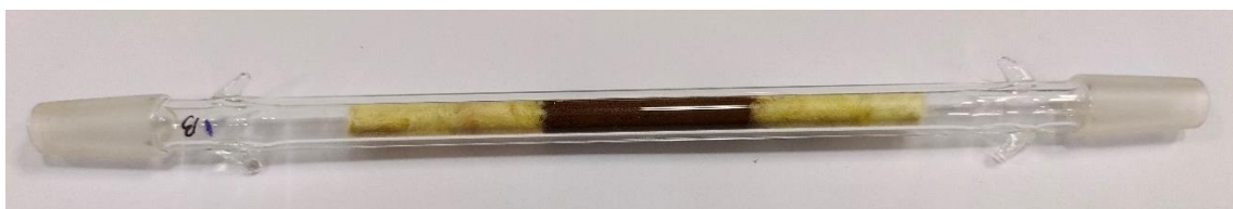
Figure 5.5: Digital image of the adsorbent column used in vapour phase dynamic \text{CH}_3\text{I} capture study.
