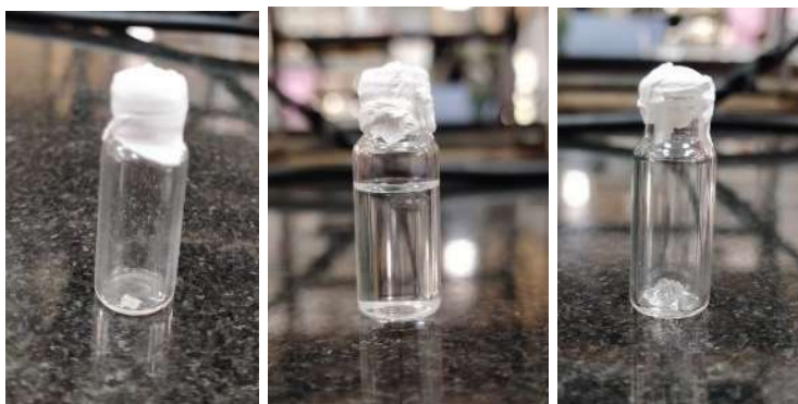
Figure 16, 17, 18 (Left to right) – Swelling of the obtained PRODET-1 in Methylene Chloride after suspension for 5 minutes. Left – Dry sample, Middle – In 1.5 mL Methylene Chloride, Right – Swollen material.
