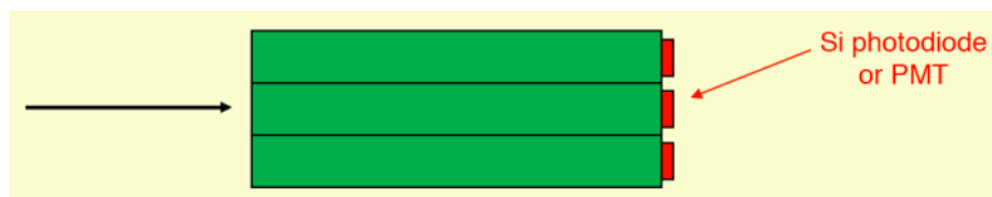
Figure 2.11: Design principle of a homogeneous calorimeter [10]
