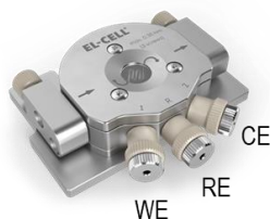
Figure 2.1: Photograph of the in-situ-electrochemical FTIR setup with \text{WO}_3 as the working electrode (WE).
