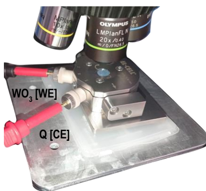
Figure 2.2: Photograph of the in-situ-electrochemical Raman setup of the battery with \text{WO}_3 as the working electrode (WE), quinone as counter electrode (CE) with WE exposed to the laser beam.
