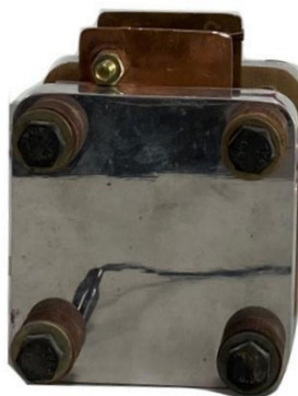
Figure 2.3: Photograph of the cell setup utilized for fabrication of the electrically rechargeable hydrogen battery and the air chargeable hydrogen battery
