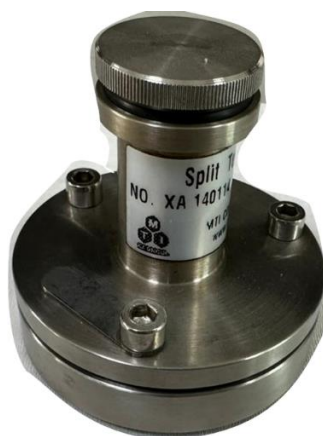
Figure 2.4: Photograph of the split cell setup utilized for the all solid state proton battery fabrication
