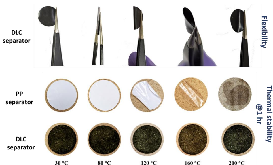
Figure 4.9: Thermal shrinkage of DLC and PP separator after heating at different temperatures for 60 min.
