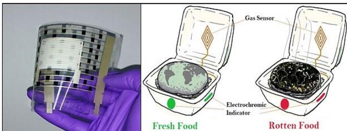
Figure 30: Ammonia sensor installed with Heater. And application in food packaging.
