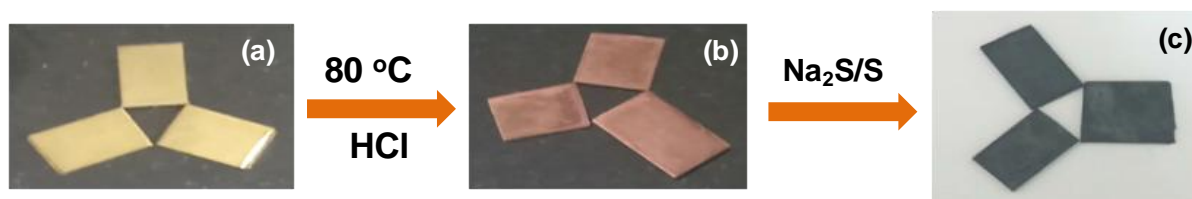
Figure 5.1: (a) Photograph of brass plate. (b) Plates after treating with HCl at 80 °C. (c) Photograph of Cu 2 S coated brass plates obtained by drop casting Na 2 S/S solution on treated brass plates shown in Figure (b).
