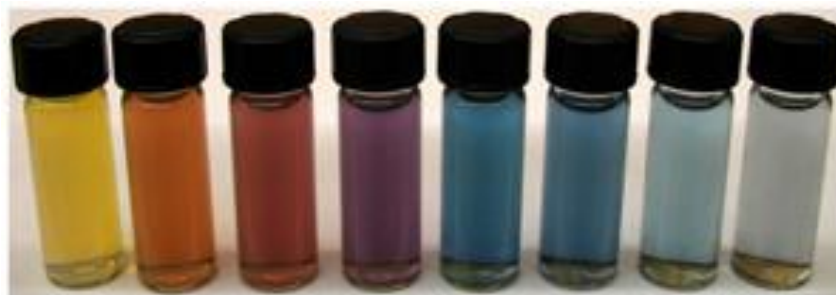
Figure 1.1 Optical photograph showing the variation in the color of gold nanorods (AuNRs) with a change in their sizes. (Adapted from reference 5)
