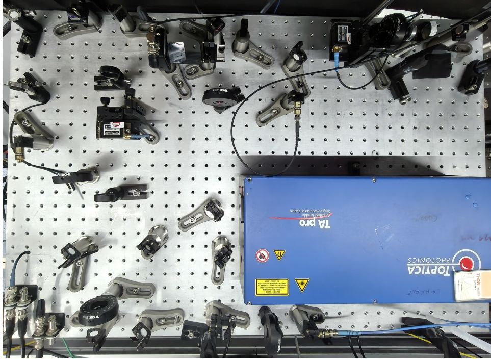
Figure 3.7: Global and single ion addressing optics for the 729 nm laser.
