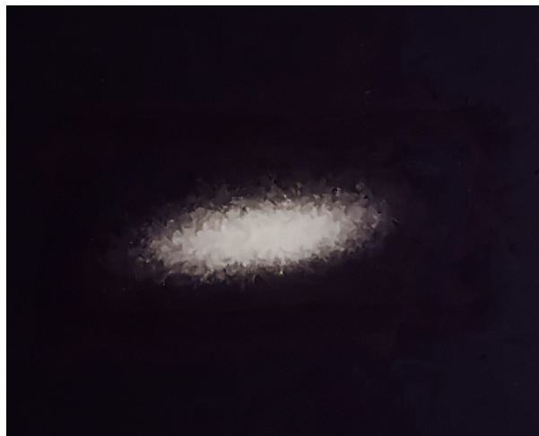
Figure 4.1: Fluorescence image of a large ion cloud containing hundreds of ions, captured by the EMCCD camera.
