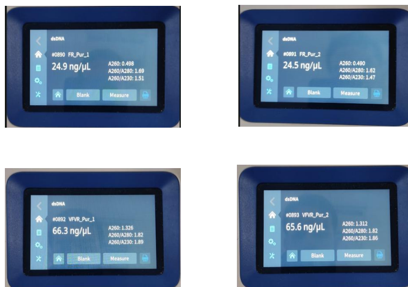
Figure 9 - NanoDrop™ readings of PCR purified products. 1 - F/R reaction; 2. F/R reaction 2; VF/VR reaction 1; and 4 - VF/VR reaction 2
