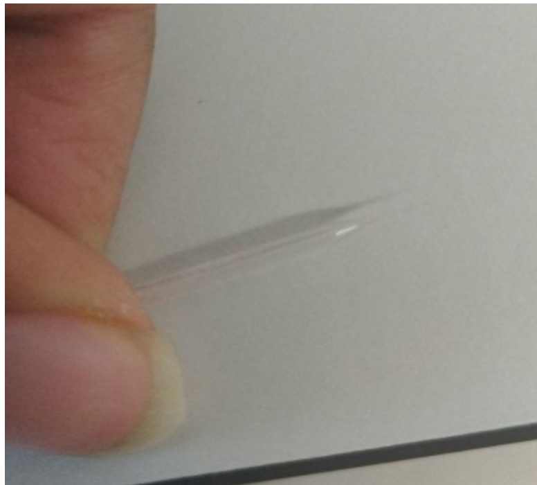
Figure 3.5 A glass needle with an extremely thin tip (~10 microns).
