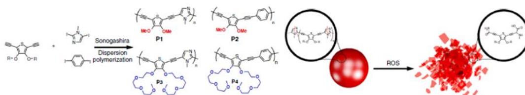
Figure 1.55. Conjugated polymer synthesis; polymerization of thiophene monomers with imidazole monomers to produce degradable polymers (P1 and P3) and polymerization with benzene monomer to obtain non-biodegradable polymers (P2 and P4) and the degradative imidazole oxidation of particle by reactive oxygen species to decompose into methyl amino acid and amide terminated 2,5-diethynylene-3,4-methoxythiophene ( adopted from Repenko et al. Nat. Commun. 2016 , 1-8)
