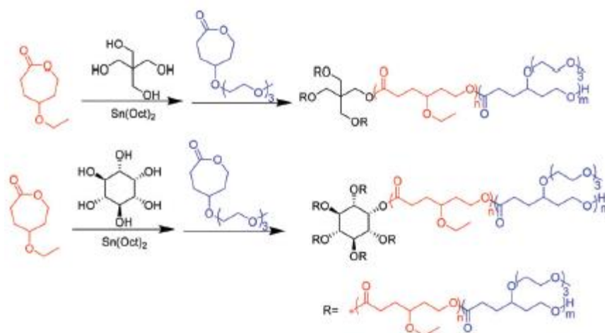
Figure 1.32. Synthesis of 4- and 6-arm star-like PECL- b -PMEEECL amphiphilic diblock copolymers (adopted from Washington et al. J. Mater. Chem. B 2017 , 5 , 5632-5640)
