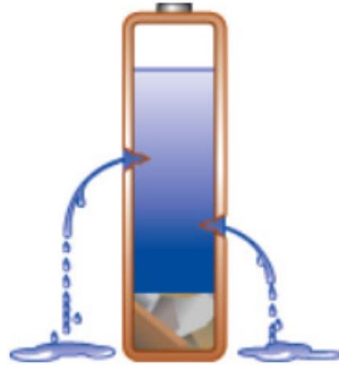
Figure 14. Self-discharge process in a battery. Reproduced with the courtesy of Isidor Buchmann, Battery University. www.batteryuniversity.com .
