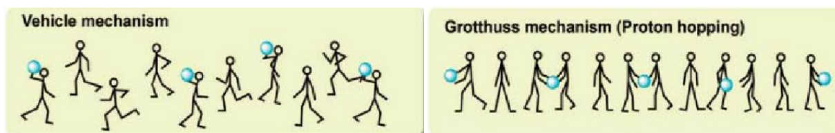
Figure 1.22. A schematic representation of the two mechanisms for the transfer of protons within a material. (Adapted from Polymers 2012, 4, 1627-1644; doi:10.3390/polym4041627)
