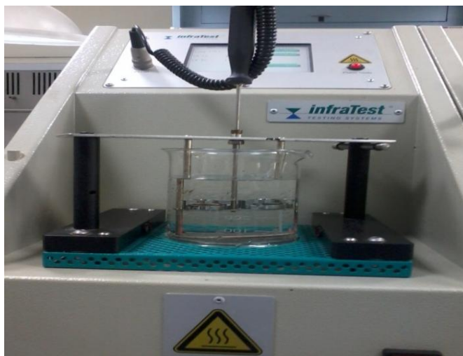
Figure 2.2.3: Infracrest 20-2200 Ring and Ball apparatus
