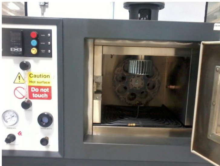
Figure 2.2.5: Koehler K88001P RTFOT instrument
