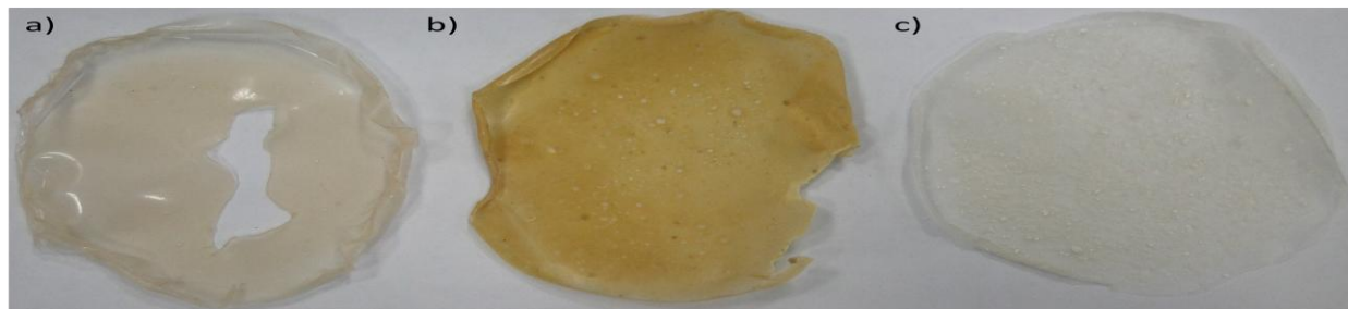
Figure 2.1.3: Image of a transparent film (after evaporation of toluene) of, a) ENR mixed with DDBS clay, b) ENR mixed with 3-ABS clay, c) ENR mixed with CO 3 clay.
