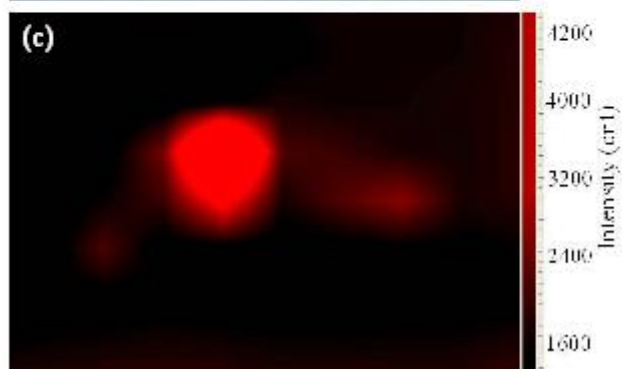
Figure 4: (a) SERS of Rh6G molecule which was coated on AgNWs, (b) An optical image which is used for Raman imaging, (c) Raman image of Ag NW shown in fig.(b). [29]
