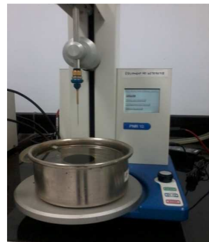
Figure 3.2.1 a: dimensions of a standard needle and Figure 3.2.1.b: Petrotest PNR-12 Penetrometer
