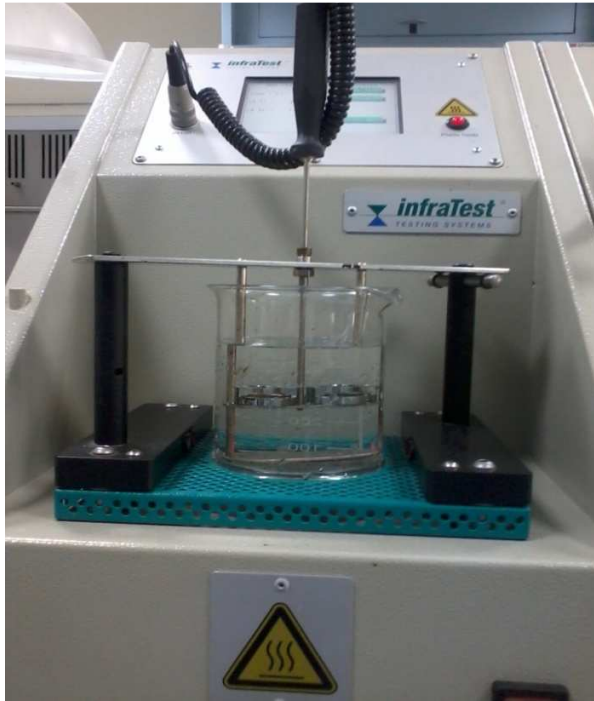
Figure 3.2.2 b: Infracast 20-2200 Ring and Ball apparatus
